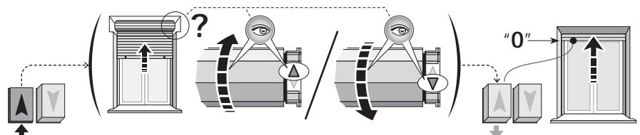
03. Lastly, memorize the level by pressing the "arrow" button identified previously all the way down (with a screwdriver) on the motor head: it **must stay down**.
